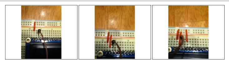
• Connect pin 1 of the display to GND, pin 2 to 5V, and pin 5 to GND.
